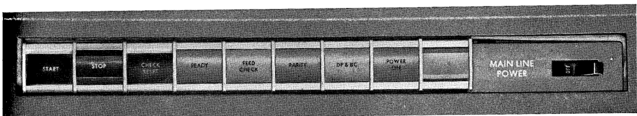
FIGURE 89. 323 PUNCH OPERATING KEYS AND LIGHTS
